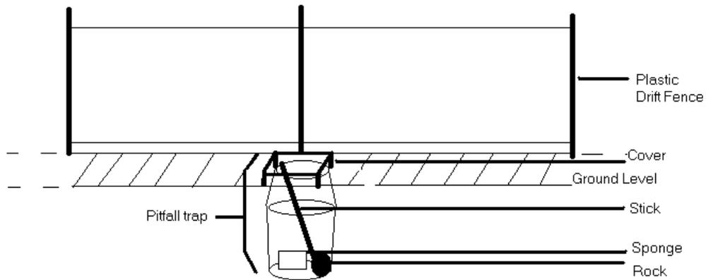
Figure 7. Diagram of a pitfall trap and drift fence used for capturing salamanders.
